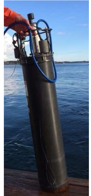
This flow cytometry allows to pass the microalgae in front of a laser beam.
