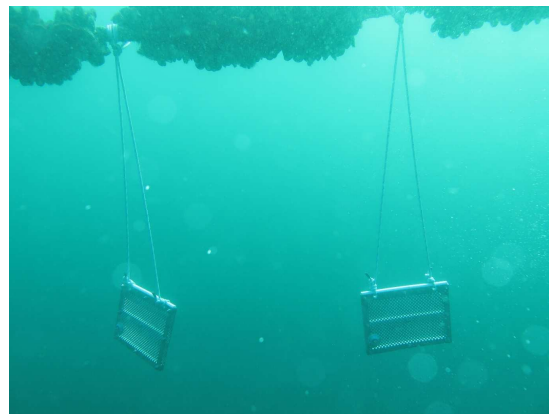
Passive sampler for contaminants in seawater deployed in the bay of Biscay. © AZTI, Ekaitz Erauskin
