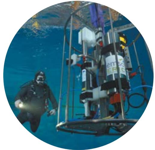
LAUNCHED IN THE FRAMEWORK OF THE EUROPEAN SEAFLOOR OBSERVATORY (EMSO), THE GENERIC INSTRUMENT MODULE (EGIM), DEVELOPED BY IFREMER, IS A STANDARDISED MEASUREMENT TOOL EMBEDDED WITH NUMEROUS SENSORS AND IS USED TO FIT SUBSEA OBSERVATION STATIONS.
