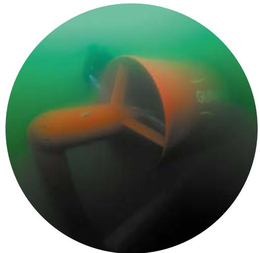
27 FEBRUARY 2019: SUBMERSION OF THE GUINARD ÉNERGIES P154 MACHINE IN THE ETEL RIA FOLLOWING POSITIVE TRIALS CONDUCTED IN JANUARY IN THE BAY OF BREST. THIS 20KW TIDAL STREAM TURBINE, DEVELOPED IN THE FRAMEWORK OF THE MEGAWATTBLUE PROJECT (GUINARD ÉNERGIES/IFREMER/ENSTA PARTNERSHIP), WAS SET UP ACCORDING TO PLAN AND WILL BE CONNECTED TO THE GRID VERY SOON. CURRENTLY, THE TURBINE IS OPERATING AND IS BEING VALIDATED.
